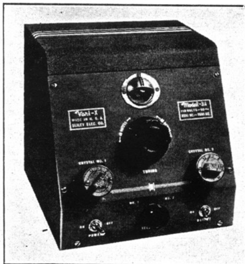
This small cabinet houses the oscillator and its power supply. The large knob at the center of the panel tunes the output circuit to either 80 or 40 meters. Crystals are plugged into the panel, where they are available for quick change or frequency shift.
